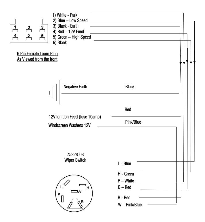
Wiper switch system is 12V Positive Feed
